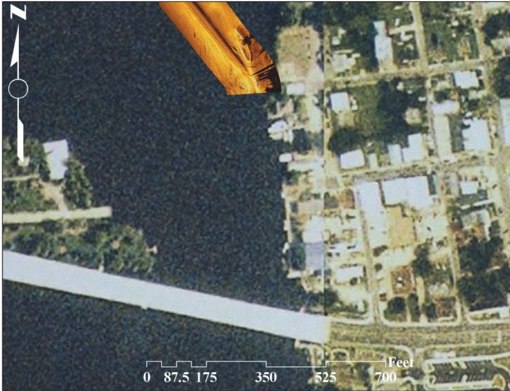
Figure 32. Georectified tile of sonar showing the location and orientation of the remains of Estelle Randall adjacent to the eastern bank of the Scuppernong River in the heart of Columbia, NC. (Image by Nathan Richards, 2011).
