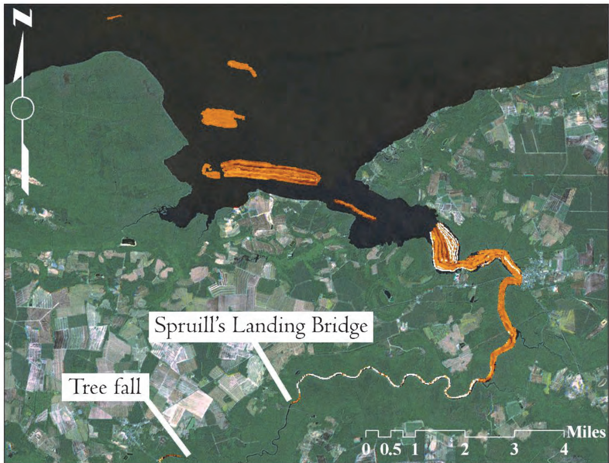
Figure 7. Total area covered during side scan surveys of the Scuppernong River and Bull Bay in 2011. Brown color indicate areas covered with the Marine Sonics 600 kHz system and white colors showing coverage with the Klein 531UT 500kHz system (Image by Nathan Richards, 2011).
