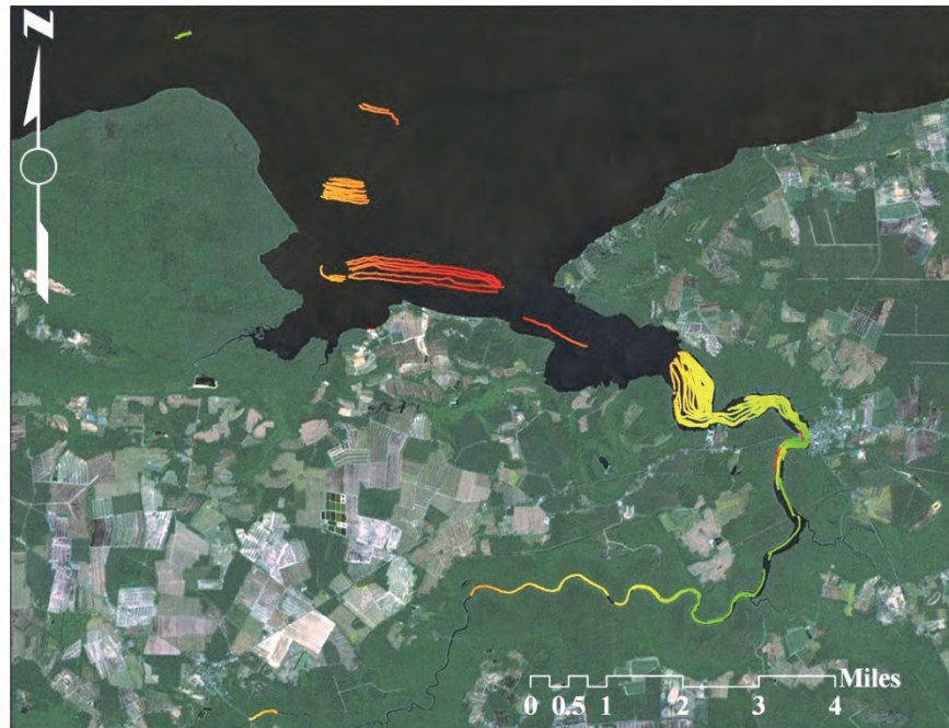
Figure 21. Survey lines traveled during magnetometer survey of the Scuppernong River and Bull Bay in 2011 (an estimation of area coverage). Colors represent nanoTesla (nT) readings from Geometrics G882 cesium magnetometer. (Image by Nathan Richards, 2011).
