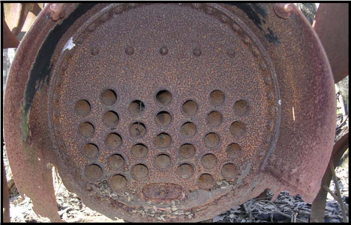
FIGURE B.16. Boiler of moveable donkey engine (photo by author 2007).
