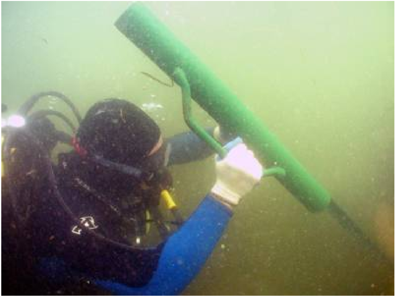
FIGURE 4.7: Diver installing a fence post used as a temporary reference point (Courtesy of the Program in Maritime Studies, East Carolina University).
