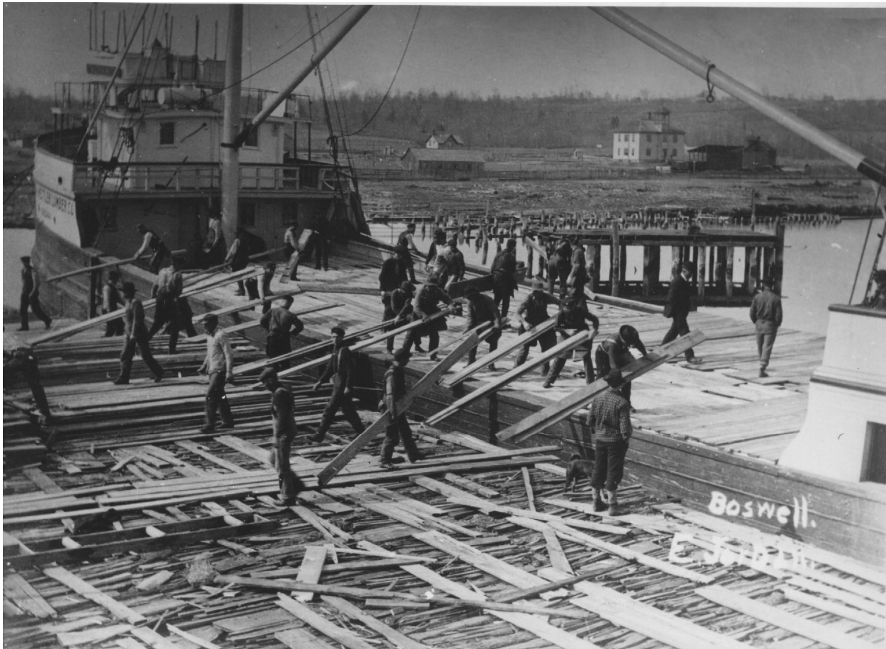
FIGURE 2.4: Lumber shovers passing lumber from the woodpile to the ship's deck (Courtesy of the C. Patrick Labadie Collection, Alpena Public Library, Alpena, Michigan).
