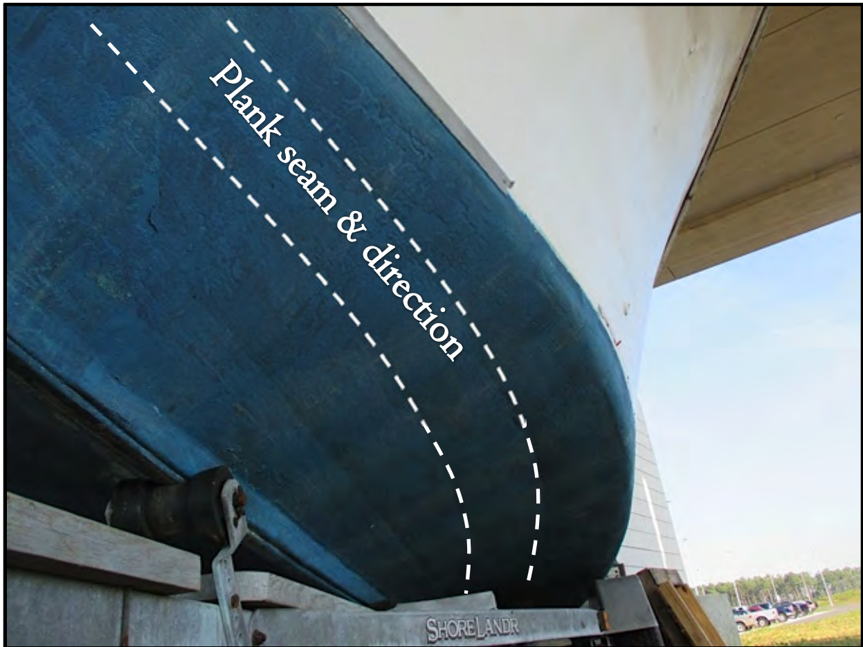
Figure 2. Fore-and-aft running hull planks (Photo by Jeremy Borrelli, 2013).
