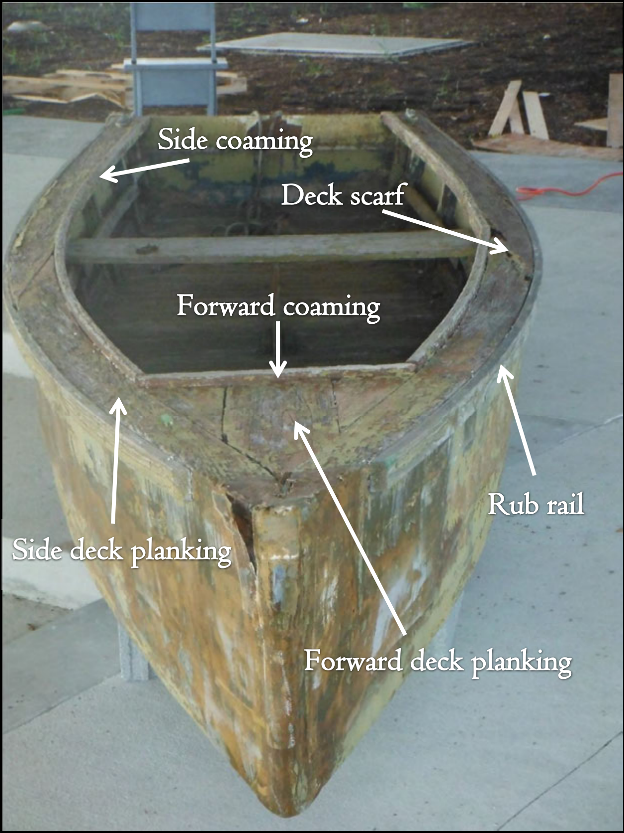
Figure 48. Forward deck, side deck, coaming, and rub rail (Photo by Ryan Bradley, 2013).
