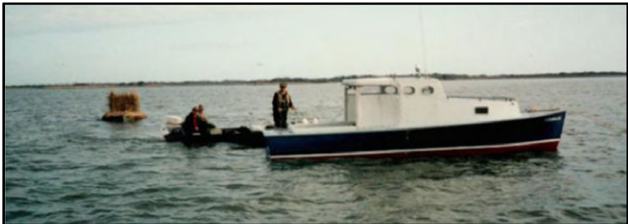
Figure 77. Image showing a tunnel boat in action tending to a hunting skiff and blind during hunting season. The boat depicted was the second concave tunnel boat built by Patrick H. O'Neal for the Bells Island Hunt Club in 1948, named Mother Goose by its second owner at Piney Island (Photo courtesy of Travis Morris).
