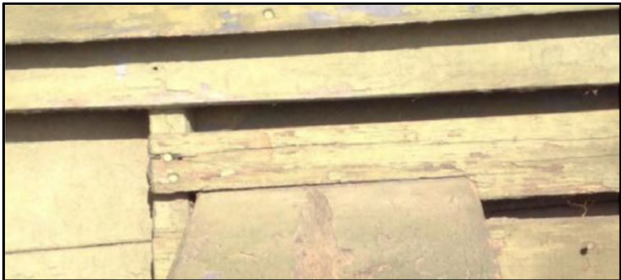
Figure 58. Thwart 3 on the starboard side showing its placement between the notched thwart support and the frame (Photo by William Sassorossi, 2013).
