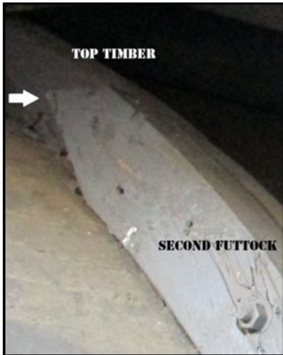
Figure 17. Image showing the beveled end of the second futtock in the second frame set (Photo by Jeremy Borrelli, 2013).
