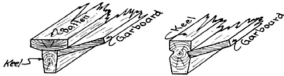
Figure 78. Image of two different types of keel potentially used when building the Slick Boat (Chapelle 1994:43).
