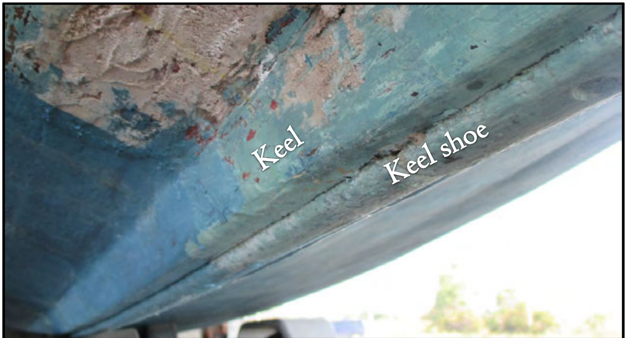
Figure 11. Keel and keel shoe, starboard side (Photo by Jeremy Borrelli, 2013).
