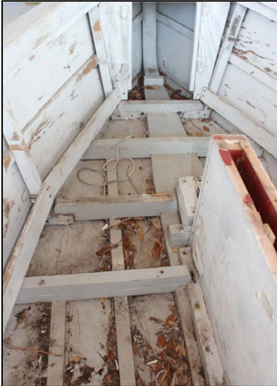
Figure 32. Bow of the vessel, including the floors, centerboard, and storage locker (Image courtesy of Caitlin Zant, 2013).
