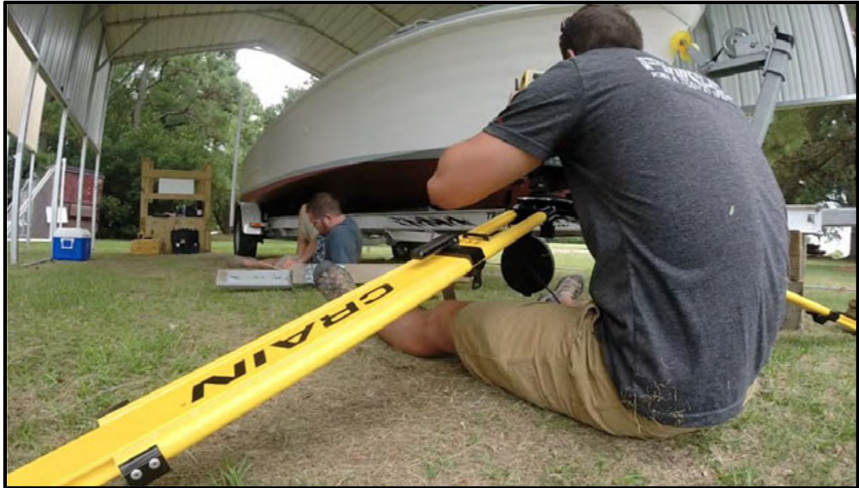
Figure 70. Photo illustrating the two-person team digitally mapping the exterior hull of the boat. Spotter Ryan Bradley catalogues the points on the hand drawings and shooter Jeremy Borrelli maneuvers the total station to the locations on the boat indicated by the spotter (Photography by Jeremy Borrelli, 2014).
