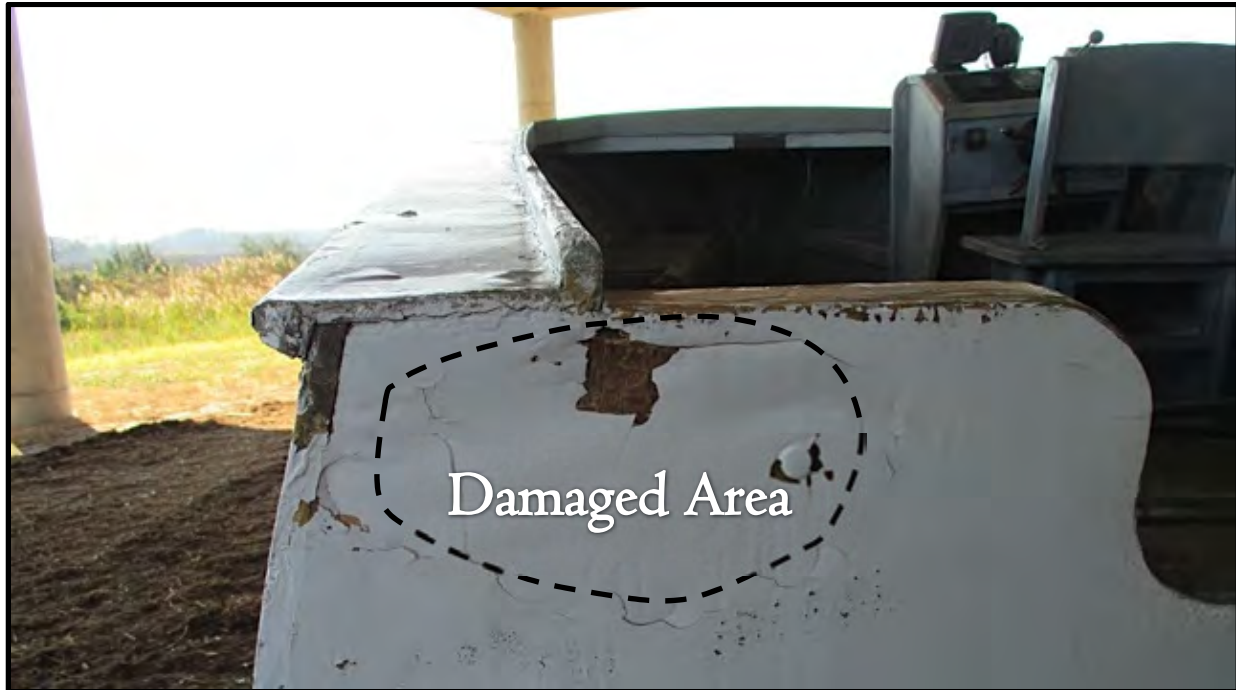
Figure 5. Repaired damage on the portside exterior of the transom (Photograph by Jeremy Borrelli, 2013).
