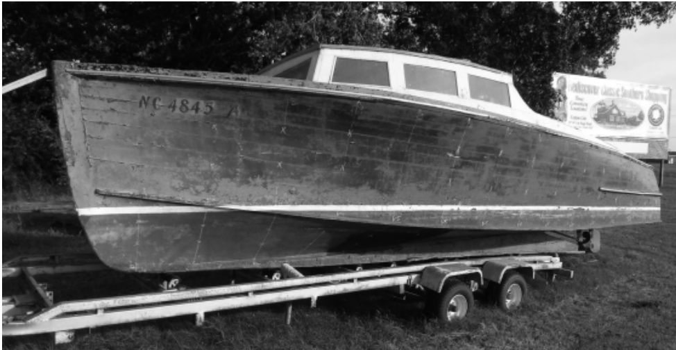
Figure 1. NCHH0025 with noted dead-rise and bow flair, Currituck, NC (Brian Diveley, 2005).
