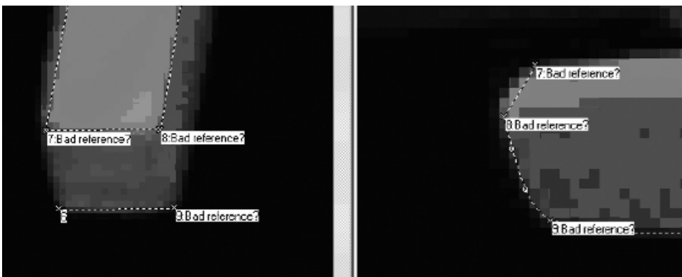
Figure 47. Three points deemed bad references because of the point of view of the photograph. The points mark the same corners, but the program, because of the photo angle, is unable to recognize that they correspond (Sami Seeb, 2005).
