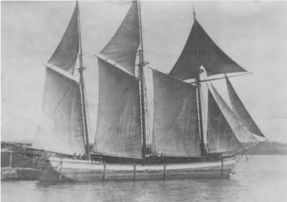
Figure 8. Dan Hayes with a full spread of canvas. Since it is still at the quay the canvas is likely set out to dry. The triangular foremast topsail is known as a rafee, and is peculiar to the Great Lakes (Courtesy of the Manistee County Museum).
