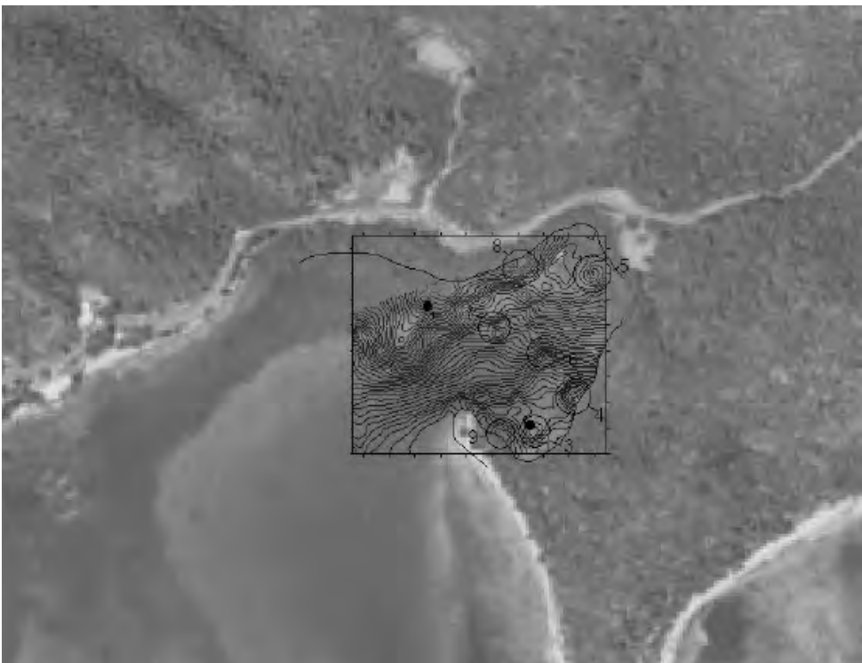
Figure 9. Magnetic anomalies and sonar targets in Borck Creek (Program in Maritime Studies, 2002).
