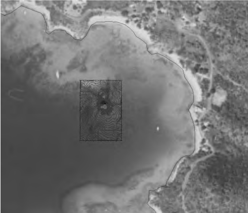
Figure 26. Magnetic signature of HMS Santa Monica (Program in Maritime Studies, 2002).
