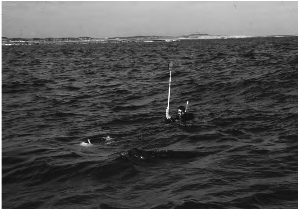
Figure 3. Frank Cantelas holds the mirror target for the Electronic Distance Meter to measure the distance from the shore datum to submerged wreck features (Program in Maritime Studies, 1996).
