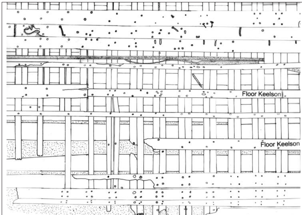
Figure 17. Detail of port side floor plan at amidships. The keelson assembly is located on the left with a single fastening pattern, and the thick strakes are located on the far right with a double fastening pattern (Courtesy Program in Maritime Studies, East Carolina University).
