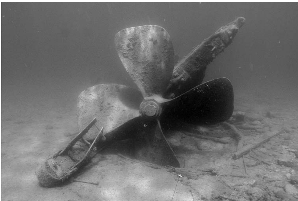
Figure 20. Photograph of Monohansett's Loper style propeller (Courtesy Program in Maritime Studies, East Carolina University).
