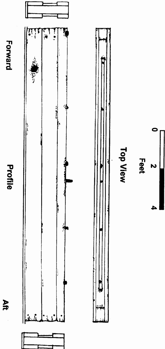
Figure 13. Centerboard trunk plan, elevation and end views. The centerboard is contained inside the trunk. Drawn by Rusty Earl.
