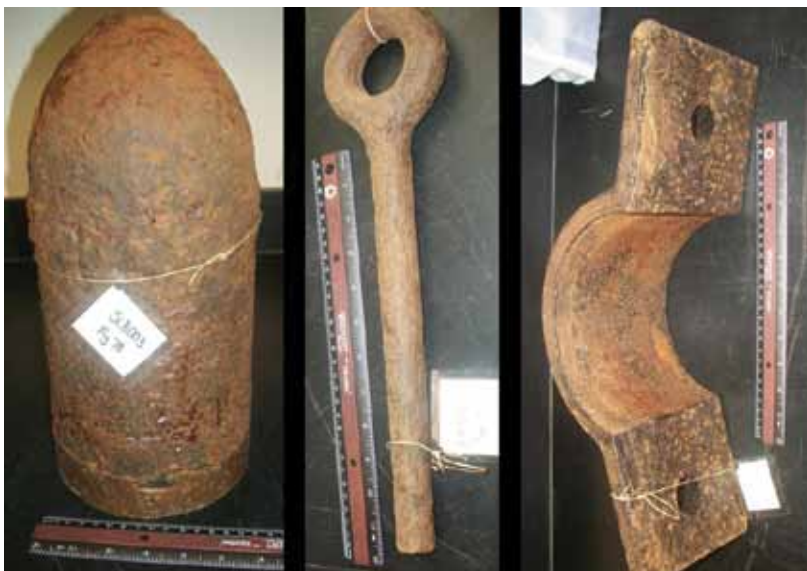
Figure 1. Examples of corroded artifacts to be conserved. From left to right: Brooke shell, wrought-iron eyehook, and trunnion cover.
