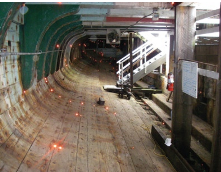
FIGURE 2: Looking aft down Wawona ’s hold. Each red dot is a point recorded with the total station.
