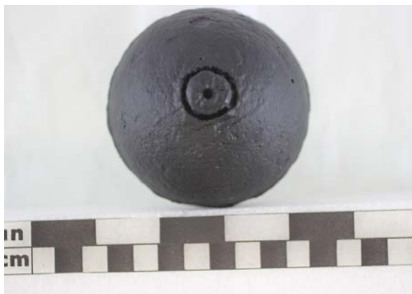
A casting spur on a grenade from Corrigan's Wreck, 1715 plate fleet.
