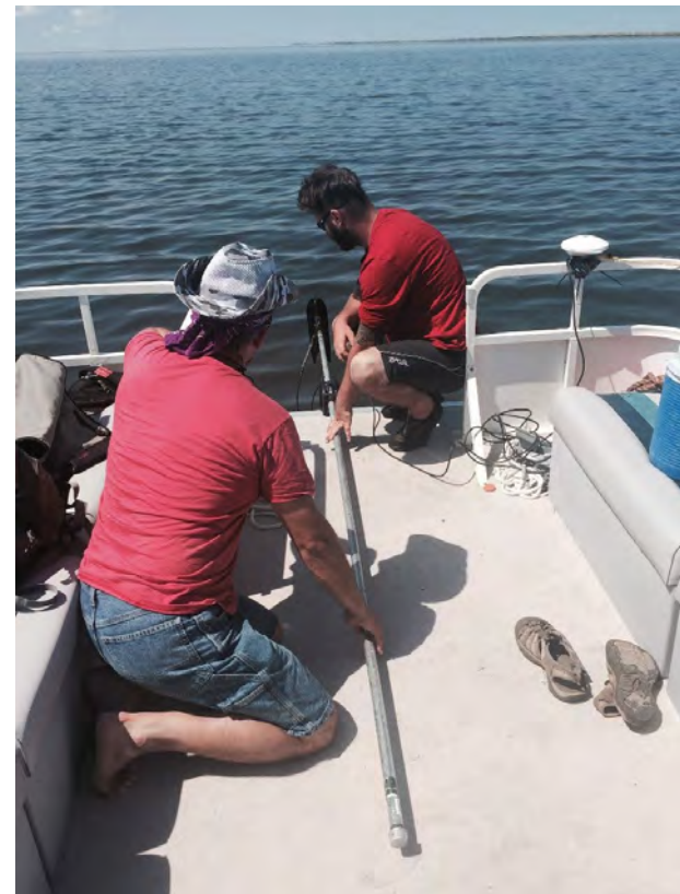
Adam Parker and Scott Rose deploying the StarFish side-scan sonar.
