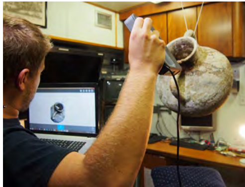
Graduate student Mateusz Polakowski 3D scanning an amphora recovered from the Egadi Islands battle site.
