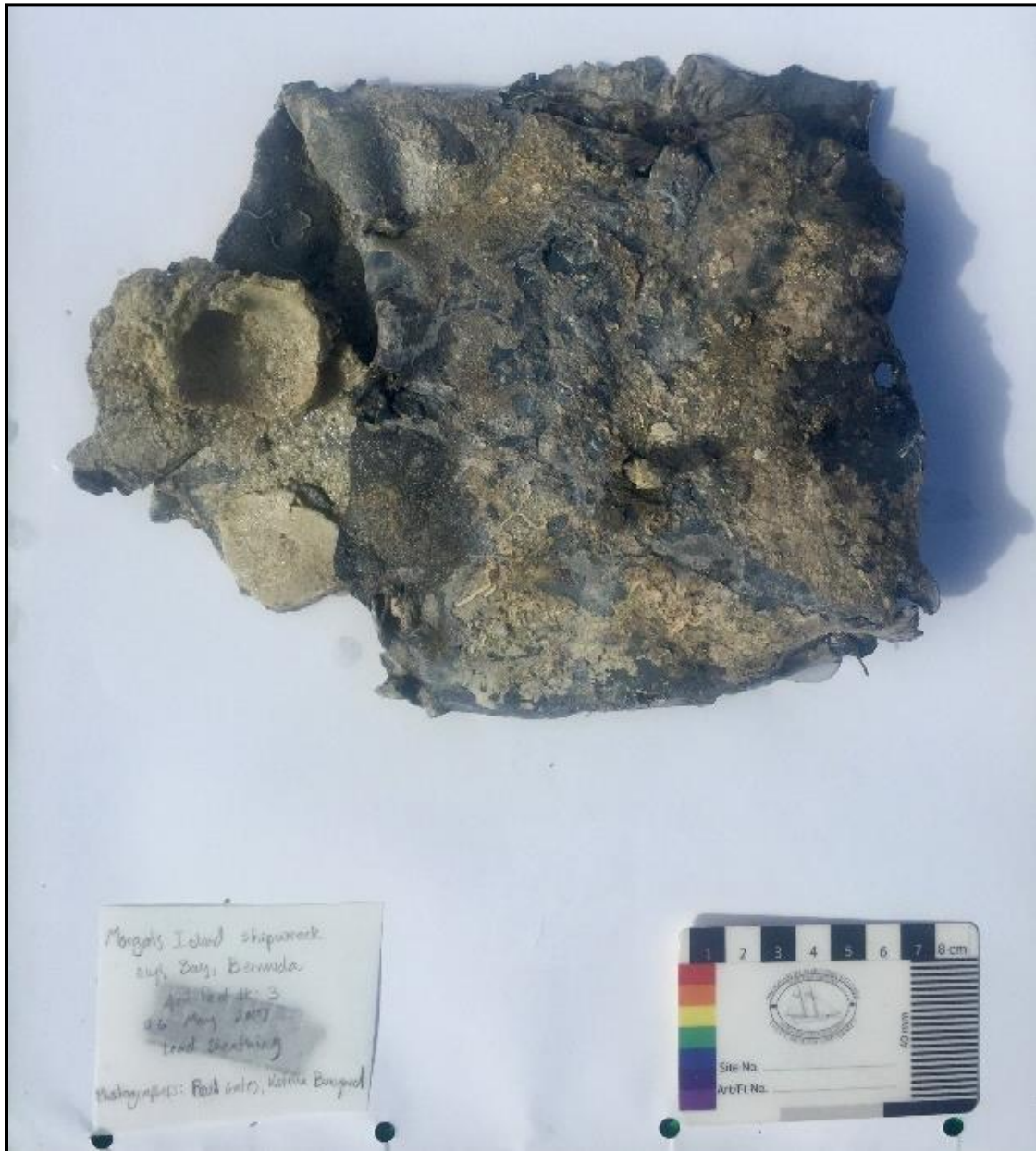
Figure 17. Folded sheet of disarticulated lead sheathing with included copper tacks recovered from the Morgan's Island Wreck site.
