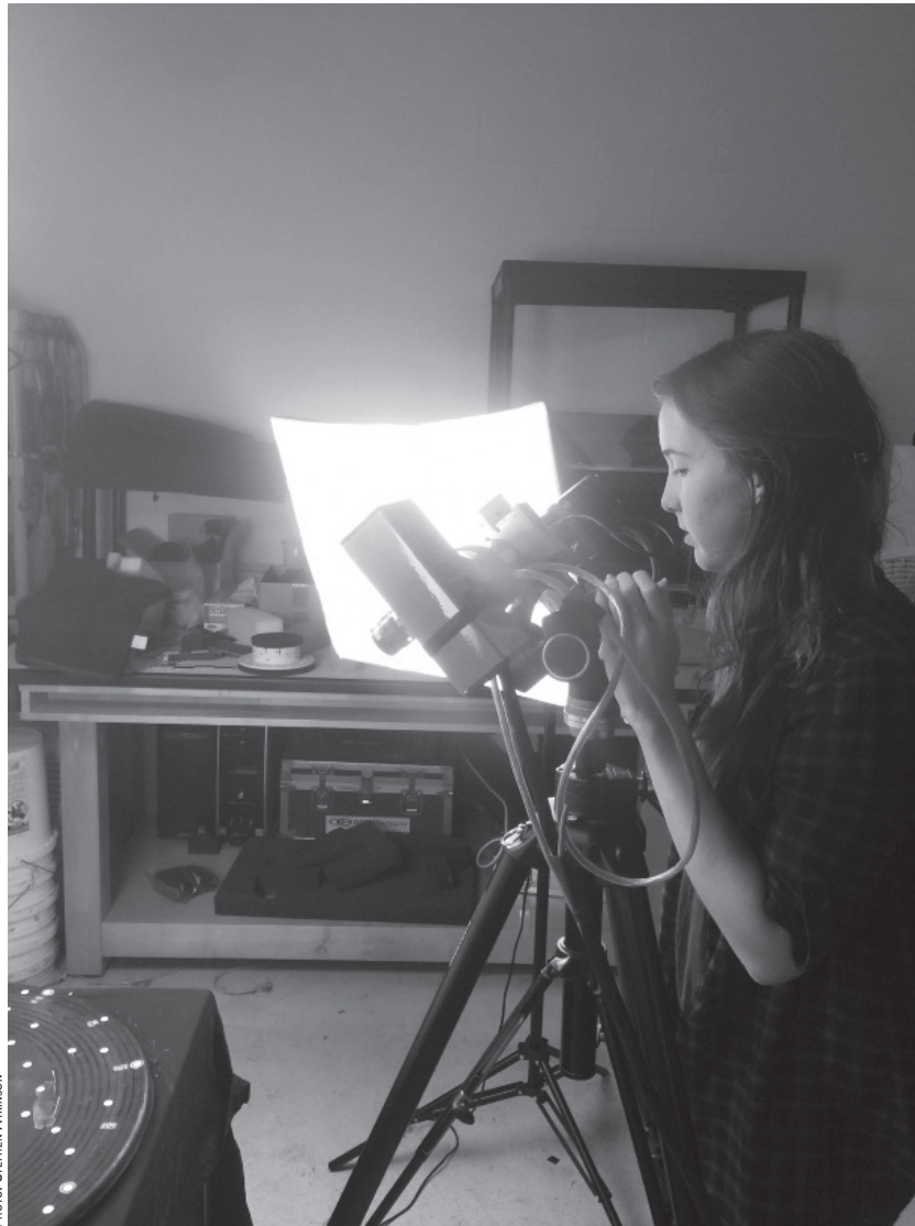
Emily Schwalbe records an artifact from the H.L. Hunley using structured light scanning.
